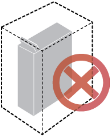
Figure 1 Inappropriately installed eAN3810A
