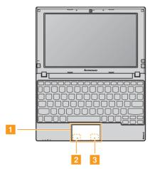
One-piece touchpad To move the cursor on the screen, slide your fingertip over the pad in the direction in which you want the cursor to move.
