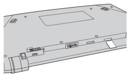
**⑤** Put the battery back in place. Turn the computer over and reconnect the cables.
