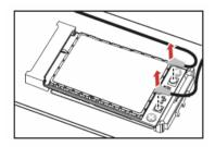
2. Remove the two screws with the screwdriver.
