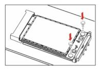
4. Insert the connector of the main antenna into the MAIN antenna interface (M) of the EM820U according to the indication on the label of the EM820U. Insert the connector of the auxiliary antenna into the AUX antenna interface (A) of the EM820U in the same way.
