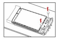
3. Slide backwards the two clips to release the EM820U from the slot. Then, lift up the EM820U.
