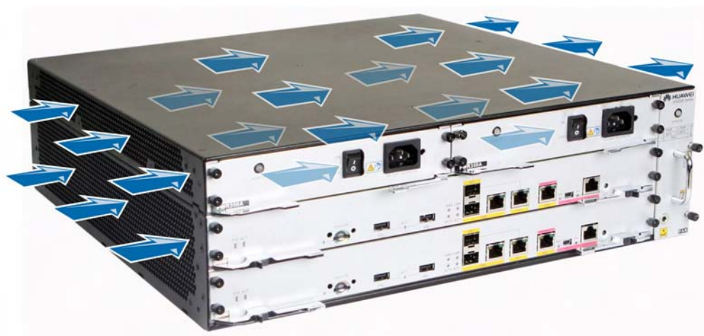
Figure 4-4 Air circulation through the AR3260 chassis
