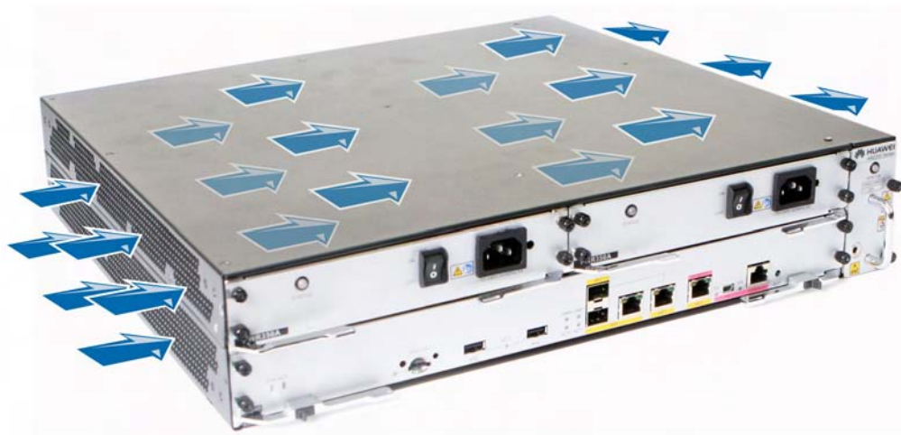
Figure 4-3 Air circulation through the AR2240 chassis
