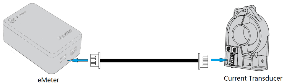
Figure 3-11 Connect eMeter with current transducer
