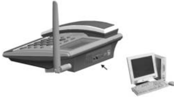
Figure 4-5 Connecting the FWT to a PC through a serial communication cable
