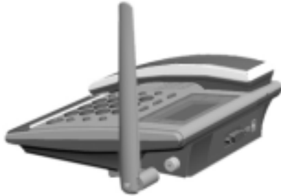
Figure 4-6 Installing an indoor antenna for the FWT
