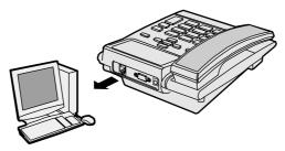
Connect the one end of the data cable to PC and the other end to the FWP. Fasten the captive screw to ensure reliable connection.
