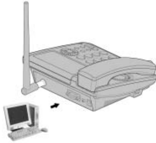
Figure 4-5 Connecting the FWT to a PC through a serial communication cable
