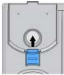
Figure 4-7 Handset retaining clip installation
