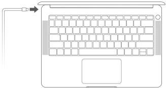
Your HONOR MagicBook has a built-in rechargeable battery, and you can charge it using the adapter and USB-C charging cable that came with it. The battery level is high or fully charged when the charging indicator stays steady white.
