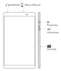
Press and hold the power key to power on or off your device or restart it.
