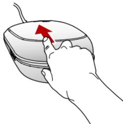
3. When the upper cover reaches the utmost front end, the **Lock/Release** button automatically locks/fixes the cover until you press it again. Now you can use the M3710 as a mouse only.
