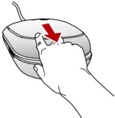
3. When the upper cover reaches the utmost rear end, the **Lock/Release** button automatically locks/fixes the cover until you press it again. Now you can use the M3710 as a mouse and a USB Modem at the same time.
