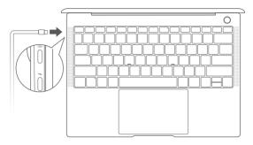
Your MateBook X Pro is pre-installed with an irremovable, rechargeable battery. You can charge your MateBook X Pro with the adapter and USB-C charging cable that comes with it. The battery is sufficiently charged when the charging indicator stays steady white.
