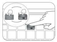
The camera button is connected to the water drainage hole on the back of your MateBook X Pro. If you accidentally spill water onto the camera, it will drain out from the drainage hole.
