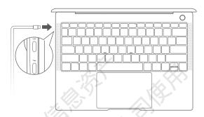
Your MateBook X Pro has a built-in rechargeable battery, and you can charge it using the adapter and USB-C charging cable that came with it. The battery level is high or fully charged when the charging indicator stays steady white.
