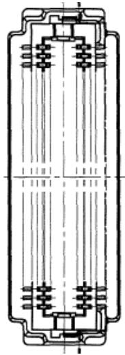
Figure 5-4 HRS DF12(3.0)-60DS-0.5V(86) connector on the MC703 CDMA EV-DO module
