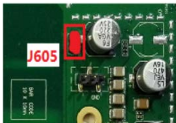
Figure 4 Jump Wire Configuration
