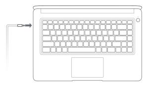
Your MateBook D Plus is pre-installed with an irremovable, rechargeable battery. You can charge your MateBook D Plus with the adapter that comes with it. The battery is sufficiently charged when the charging indicator stays steady white.
