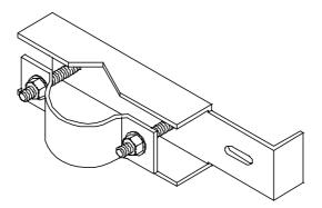
Figure 3-2 Omni antenna fixing clip (1)
