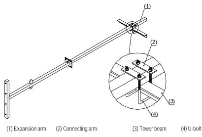
Figure 3-14 Installing the antenna support on tower
