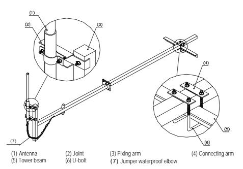
Figure 3-23 Installing the omni antenna
