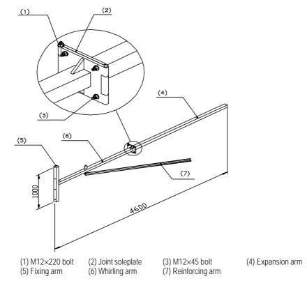
Figure 3-12 Structure of antenna support installed on tower
