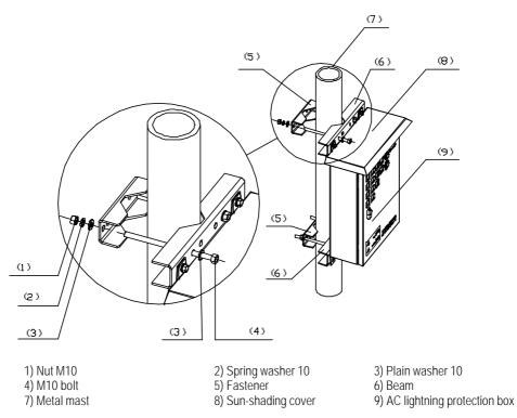
Figure 2-38 Fixing AC lightning protection box (on metal masts)
