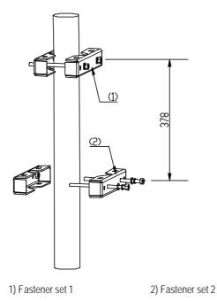
Figure 2-18 Installing fastener sets
