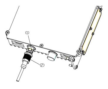
1) Fixing the limit pivoted arm into the locating slot2) External nutFigure 2-28 Installing waterproof fiber (2)
