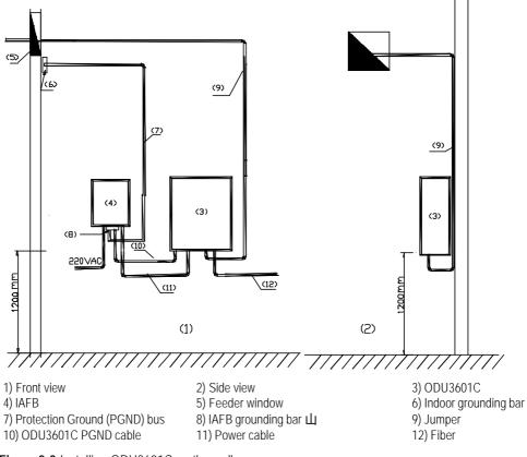
Figure 2-3 Installing ODU3601C on the wall
