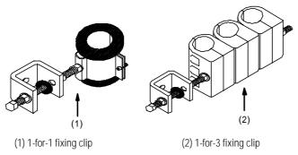
Figure 3-36 Feeder fixing clip
