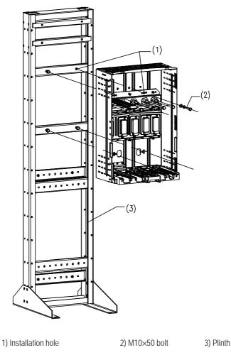
Figure 2-17 Securing rack onto plinth
