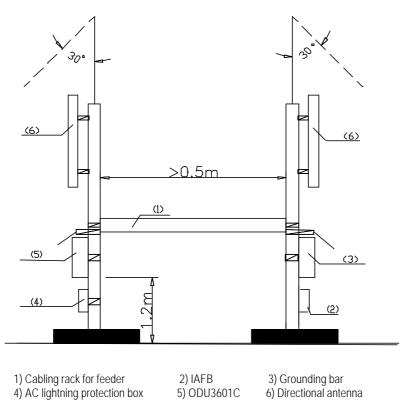
Figure 2-7 Directional ODU3601C installation on metal masts
