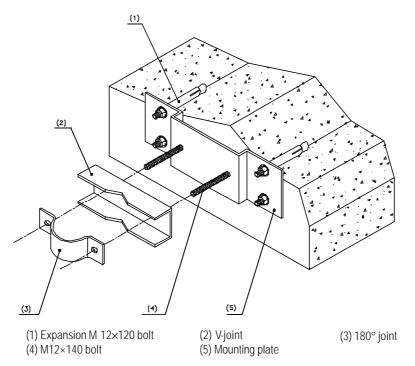
Figure 3-18 Fixing clip of antenna support installed on parapet
