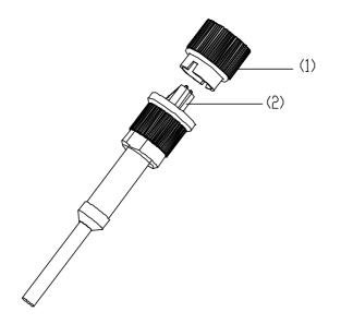
1) Dustproof cover 2) Dual-LC fiber connector **Figure 2-25** Appearance of waterproof fiber (figure 1)
