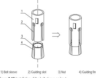
Figure 2-12 Installation of the bolt sleeve and nut
