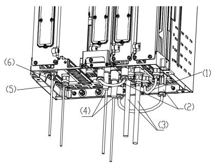
1) Inter-module cables between<br/>Type N male connectors2) Cables connecting Type D connectors3) Antenna feeder DIN connector<br/>connecting to feeder4) MTRM fiber cascading connector5) AC power input cable6) DC input power cable of battery
