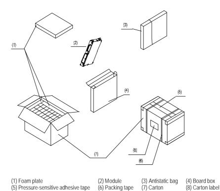
Figure 1-2 Unpacking of the module
