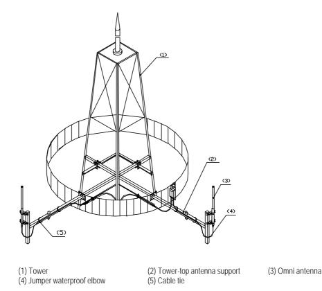
Figure 3-22 Installing the omni antenna on tower platform
