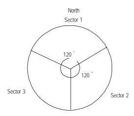
Figure 3-26 Correspondence between directional antenna azimuth and sector
