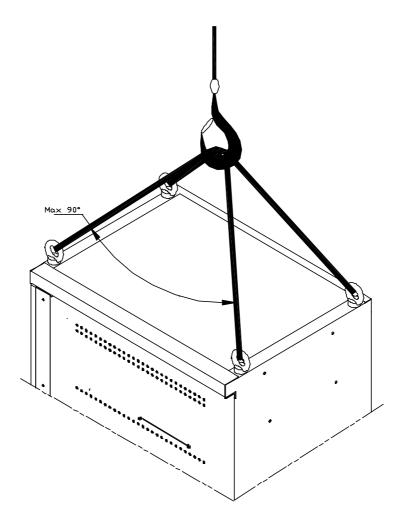
Figure 6 Hoisting of the heavy objects
