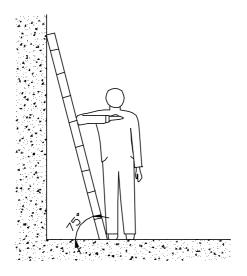
Figure 2 The angle at which the ladder should be leaned
