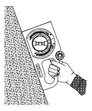
Figure 3-28 Pitch angle of the antenna after being adjusted by the inclinometer
