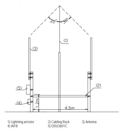
Figure 2-6 Omni ODU3601C installation on metal masts
