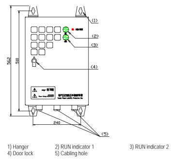
Figure 2-33 AC lightning protection box appearance
