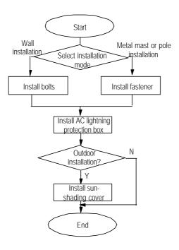
Figure 2-34 Installation flow of AC lightning protection box
