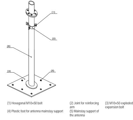
Figure 3-16 Installing the antenna support base
