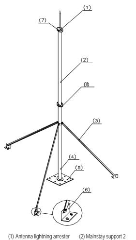
(3) Reinforcing arm (4) Mainstay support 1 (6) Anchor of reinforcing (7) Soldered parts (8) M10×80 bolt
