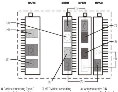
connectors between modules. 4) Inter-module cable between Type N male connectors 7) DC input power cable of battery
