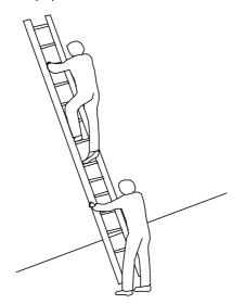
Figure 4 Climbing and using the long ladder in a safe way
