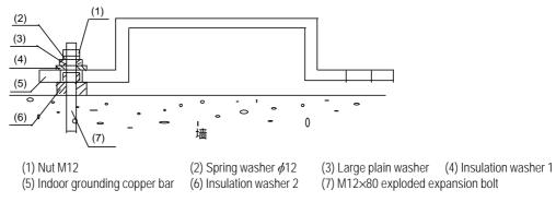
Figure 3-10 Sectional view of grounding copper bar installation
