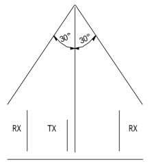
Figure 3-13 Installing the lightning arrester
