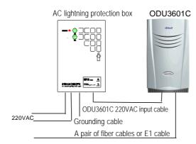
Figure 2-48 Networking of AC lightning protection box (20kA, without the IABB)
