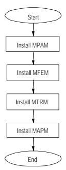
Figure 2-21 Module installation flow
