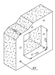
Figure 3-32 Mounting holes for feeder window
