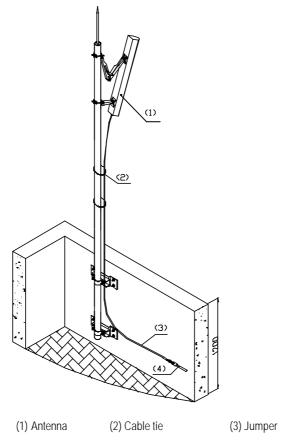
Figure 3-30 Installing the directional antenna on building-top support (with parapet not shorter than 1200mm)
