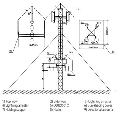
Figure 2-8 Installing ODU3601C on tower
