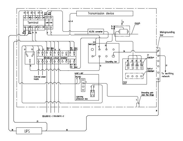
Figure 2-55 Cable distribution in IAFB networking
