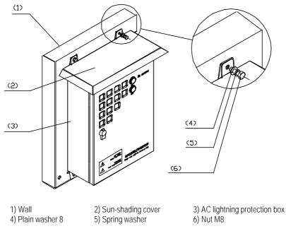
Figure 2-36 Installing sun-shading cover for AC lightning protection box
