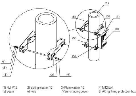
Figure 2-39 Fixing AC lightning protection box (on pole)
