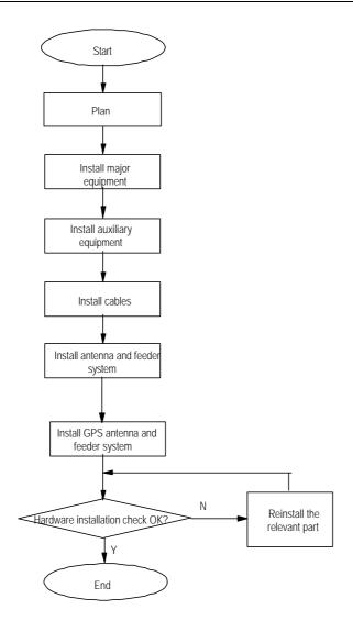
Figure 2-2 Hardware installation flow
