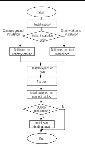
Figure 2-41 Installation flow of the IABB
