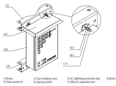
Figure 2-37 Fixing the box on beams
