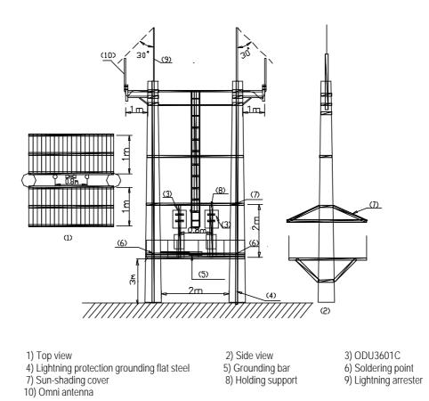
Figure 2-5 Installing ODU3601C on two poles
