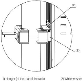
Figure 2-19 Fixing rack with fasteners
