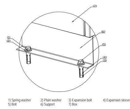
Figure 2-43 Fixing the box onto the concrete floor
