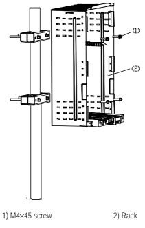
Figure 2-20 Fixing the rack
