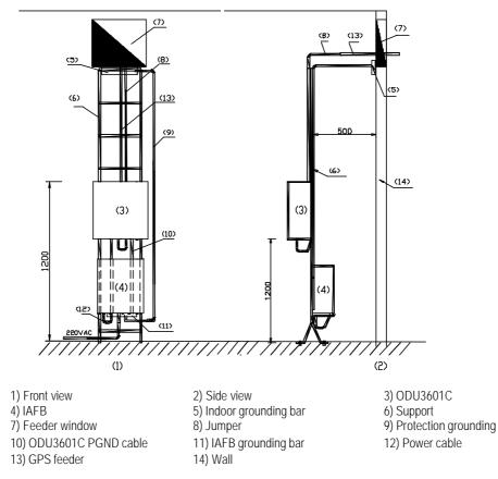
Figure 2-4 Installing ODU3601C on the plinth
