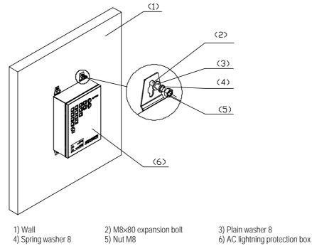
Figure 2-35 Fixing AC lightning protection box (on wall)
