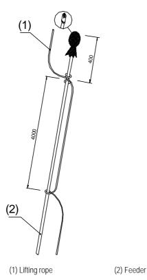
Figure 3-34 Protection of feeder connector
