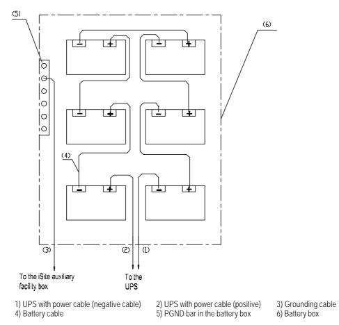
Figure 2-44 Connecting UPS to the IABB
