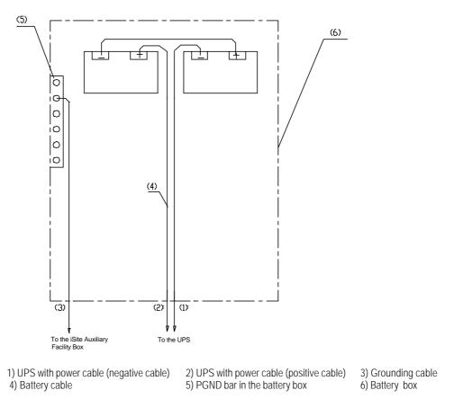
Figure 2-45 Internal connection of the IABB (without UPS)
