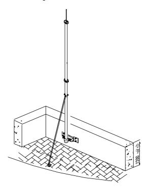
Figure 3-20 Antenna support fixed on parapet (with parapet shorter than 1200MM)
