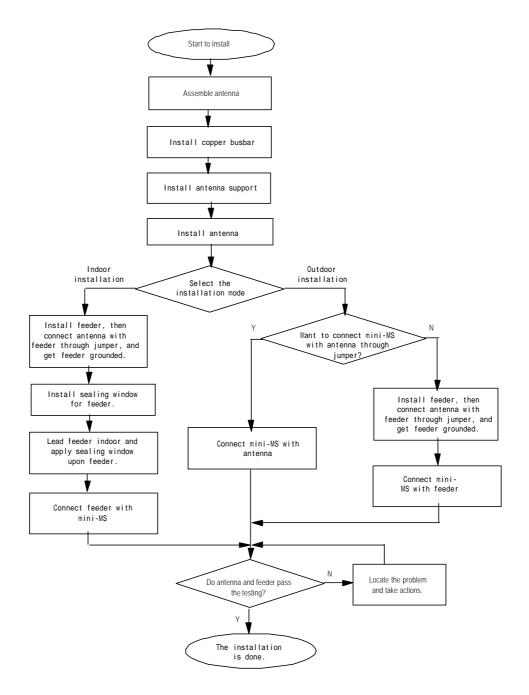
Figure 3-1 Installation flow of antenna and feeder system
