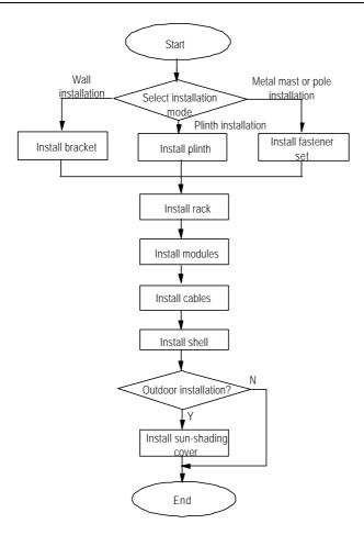
Figure 2-9 ODU3601C major equipment installation flow
