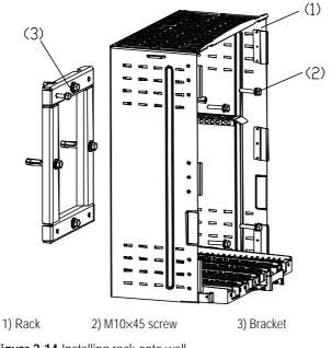
Figure 2-14 Installing rack onto wall
