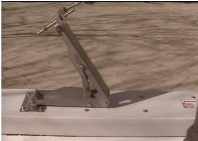
Figure 3-6 Directional antenna tilt angle adjustment device
