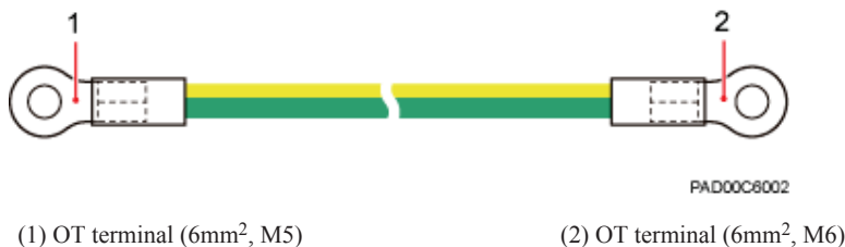
Figure 14-39 Exterior of a PGND cable
