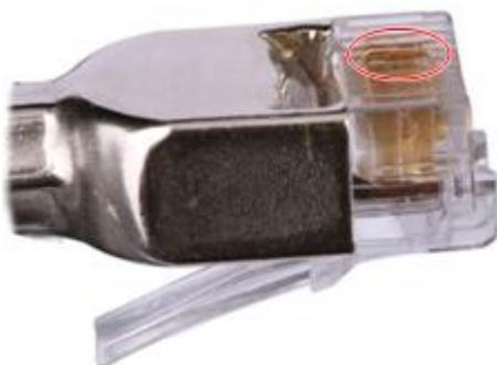
**Step 3** Check whether the contact strips are clean. If they are not clean and the dirt cannot be removed, replace it with a new RJ45 connector. **Figure 5-35** shows an unqualified piece.
