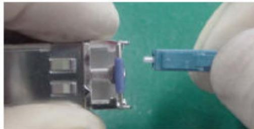
3. Cover unused optical connectors with protective caps, as shown in [Figure 5-99](#), and then lay out fibers on the fiber rack or coil them in a fiber management tray to prevent fibers from being squeezed.
