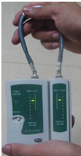
The procedure for testing a crossover cable is the same as that for testing a straight-through cable except for the sequence in which the indicators turn on, which depends on the wire connections of a crossover cable.
