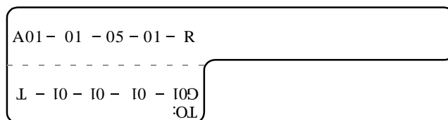
Figure 5-89 Sample label on an optical fiber between two devices
