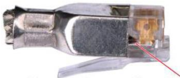
Figure 5-37 Wires not in good contact with the edge of the RJ45
