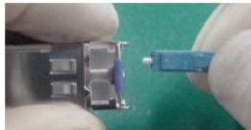
Figure 5-98 Using fibers to protect an optical module
