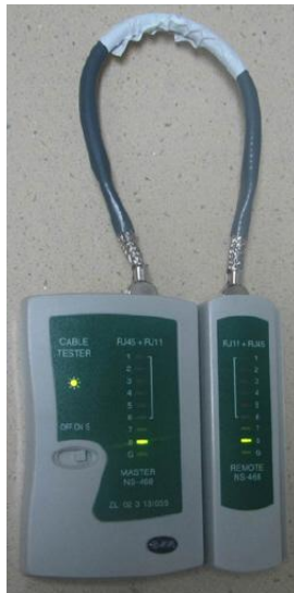
Figure 5-39 Testing the conduction and connections of wires
