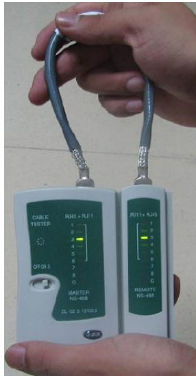
Figure 5-40 Checking the reliability
