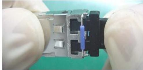
Figure 5-97 Installing a protective cap
