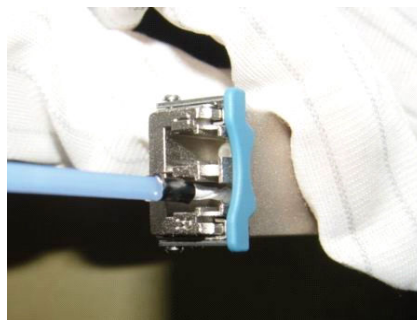
Figure 5-100 Cleaning a receptacle with a cotton swab
