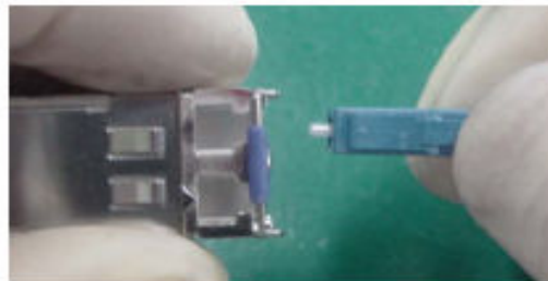
Figure 5-98 Using fibers to protect an optical module
