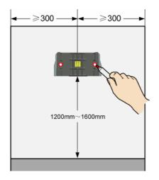
2 Drill holes at the anchor points and then install the expansion bolt assemblies.
