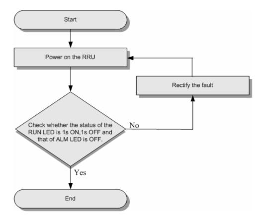
The RRU should be powered on in 24 hours after being unpacked. The power off duration of the RRU cannot exceed 24 hours during maintenance.
