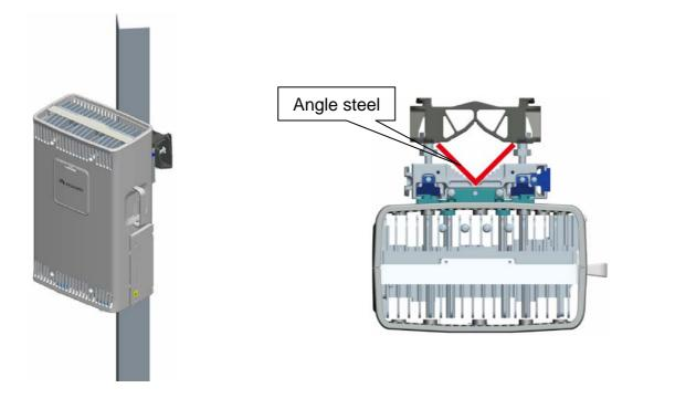
The procedure for installing the RRU on an angle steel is the same as that for installing the RRU on a metal pole.
