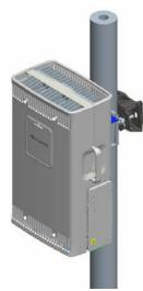
Install the main fixture of another RRU. Ensure that the main and auxiliary fixtures are perfectly fitted.
