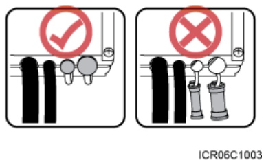
Figure 8-21 Correct placement of waterproof blocks
