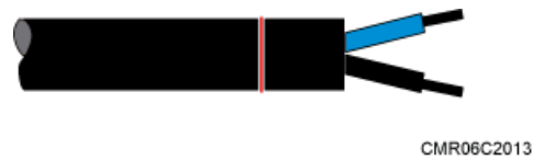
Figure 11-4 Stripping the sheath off each core wire
