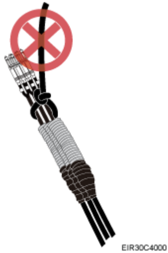
Figure 6-6 Incorrect binding method
