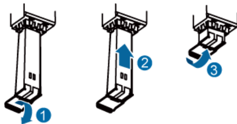
Figure 7-19 Installing an optical module
