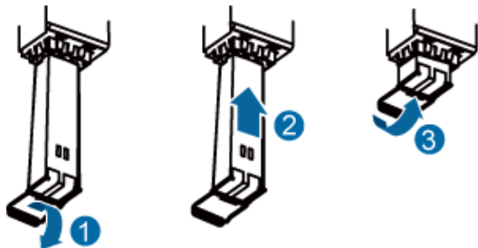
Figure 7-24 Installing an optical module
