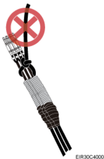
Figure 6-8 Incorrect binding method
