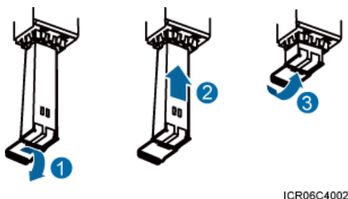
Figure 8-22 Installing an optical module
