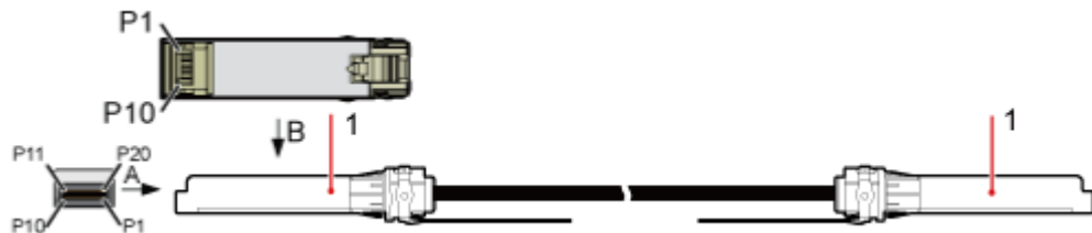
Figure 3-9 SFP high-speed cable for cascaded RRUs
