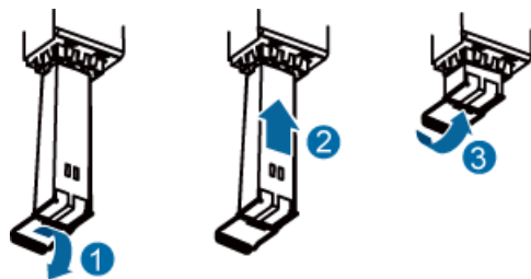
Figure 9-22 Installing an optical module
