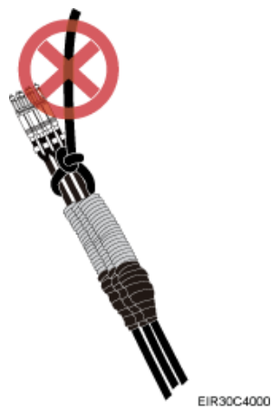
Figure 7-8 Incorrect binding method
