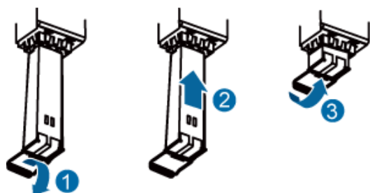
Figure 9-26 Installing an optical module
