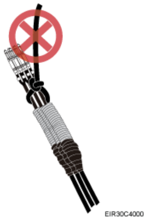
Figure 7-8 Incorrect binding method
