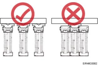
Figure 3-17 Correct installation of mounting brackets for multiple RRUs installed on an indoor wall in side-mounted mode
