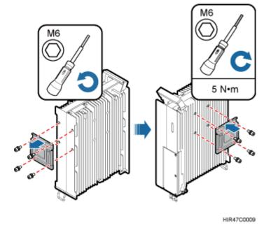
Figure 8-24 Installing the attachment plate onto the rear of the RRU
