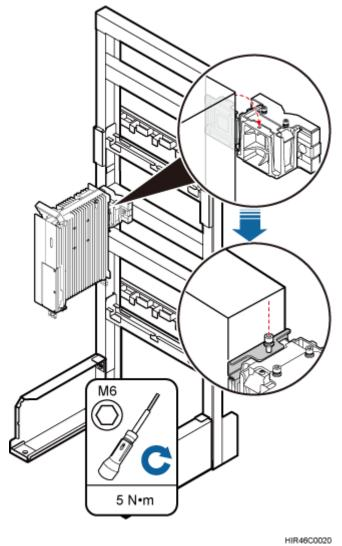
Figure 8-46 Installing the RRU onto the main bracket
