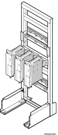
Step 6 Optional: When the ambient temperature is equal to or higher than the lowest operating temperature of the RRU and at least 10°C (10°F) lower than the highest operating temperature of the RRU, repeat the preceding steps to install the RRUs on the higher level, as shown in Figure 8-48.
