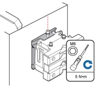
Figure 8-26 Securing the captive screw into the connection hole
