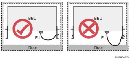
Figure 9-3 E1 cables routed through the cabinet
