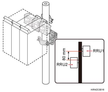
Step 6 Install the fourth RRU onto the fourth main bracket, use an inner hexagon torque screwdriver to tighten the captive screw into the holes of the attachment plate and main bracket to 5 N·m (44.25 lbf·in.) so that the attachment plate and main bracket are firmly secured, as shown in Figure 8-19.
