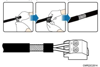
Figure 12-8 Stripping the sheath off the power cable
