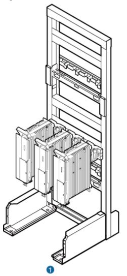
Figure 3-20 Three RRUs installed on an IFS06
