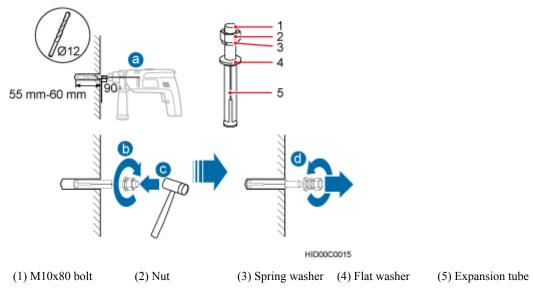
1. Use a hammer drill with a  $\Phi$ 12 bit to drill holes vertically at the marked anchor points. Ensure that the depth of each hole ranges from 55 mm (2.17 in.) to 60 mm (2.36 in.).
