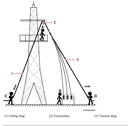
Figure 7-6 Hoisting fiber optic cables onto the tower
