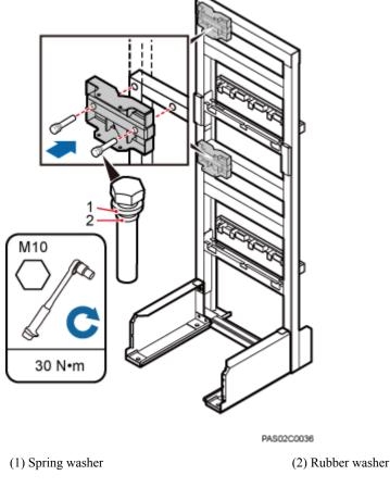
Figure 8-44 Installing the pole installation bracket in height-unrestricted scenarios
