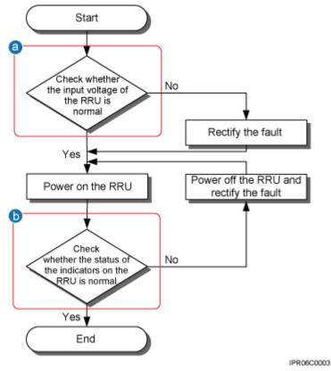
(a) The normal input voltage of an RRU is -48 V DC. The voltage of the external power supply should range from -36 V DC to -57 V DC.
