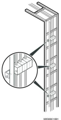
Secure cables on the tower, as shown in Figure 9-2.
