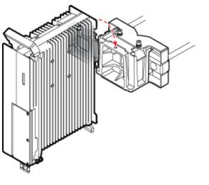
Figure 8-6 Installing the RRU onto the main bracket
