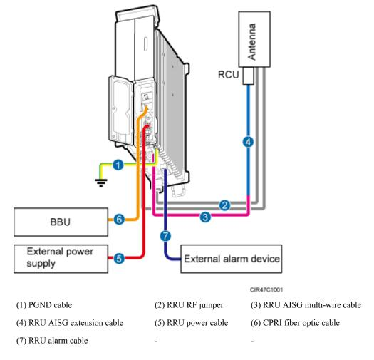
Figure 9-7 Cable connections for a single RRU
