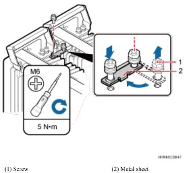
Figure 8-17 Installing the metal sheet
