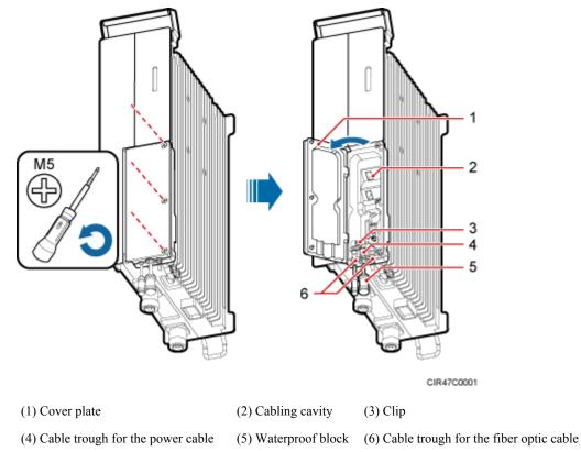
Step 3 Loosen the screws on the clip, and open the clip, as shown Figure 9-20.
