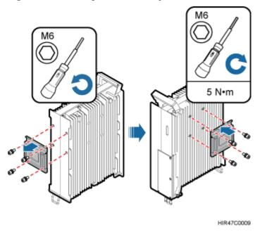
Step 5 Install the RRU onto the main bracket, as shown in Figure 8-32.
