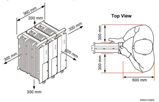
Figure 3-27 Minimum clearances for multiple RRUs installed in centralized mode
