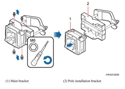
**Step 3** Install the third main bracket and install the third RRU onto the third main bracket. Then use an inner hexagon torque screwdriver to tighten the captive screw into the connection holes on the top of the attachment plate and main bracket for the RRU, with a torque of 5 N·m (44.25 lbf·in.), as shown in **Figure 8-16**.
