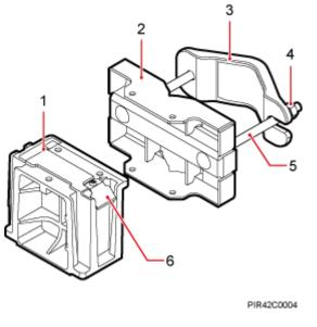
(1) Main bracket (2) Pole installation (3) Auxiliary bracket (4) Nut (5) Square-neck bracket
