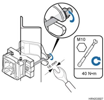
Figure 8-30 Securing the RRU mounting brackets
