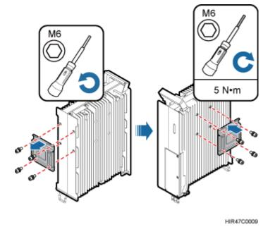
Figure 8-39 Installing the attachment plate onto the rear of the RRU
