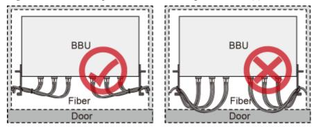
Figure 9-4 CPRI fiber optic cables routed through the cabinet (1)
