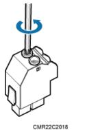
2. Connect the blue core wire labeled NEG(-) to the - port and the black/brown core wire labeled RTN(+) to the + port on the tool-less female connector (pressfit type), and then tighten the screws using a Phillips screwdriver, as shown in **Figure 12-7**.
