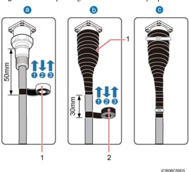
Figure 9-13 Waterproofing a connector of the RF jumper
