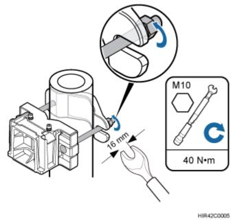
Figure 8-5 Securing the RRU mounting brackets
