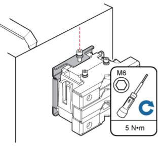
Figure 8-41 Securing the captive screw into the connection hole
