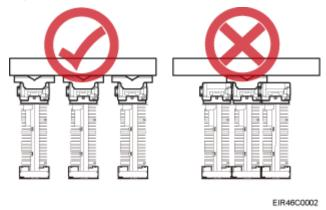
Figure 3-20 and Figure 3-21 show RRUs installed on an IFS06.
