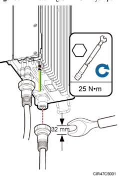
Figure 9-12 Installing an RRU RF jumper
