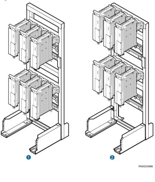
Figure 3-21 Six RRUs installed on an IFS06
