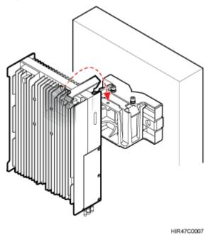
Figure 8-40 Installing the RRU onto the main bracket
