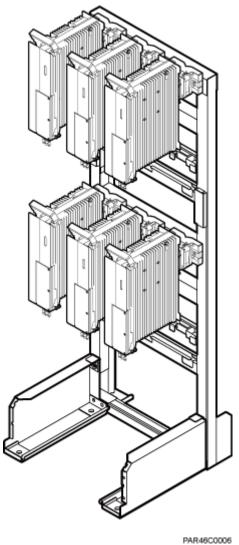
Figure 8-48 Installing RRUs on the higher level
