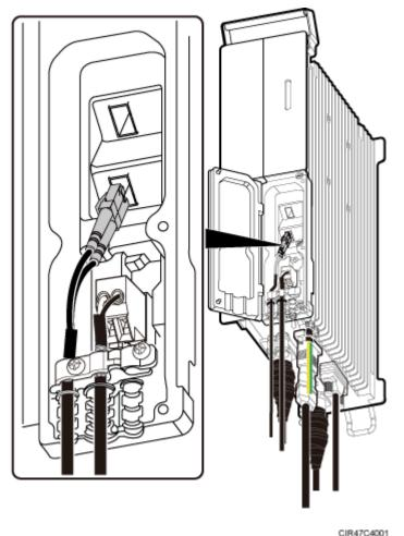
Figure 9-23 Installing a CPRI fiber optic cable
