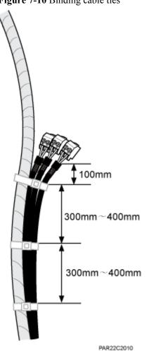
Figure 7-10 Binding cable ties
