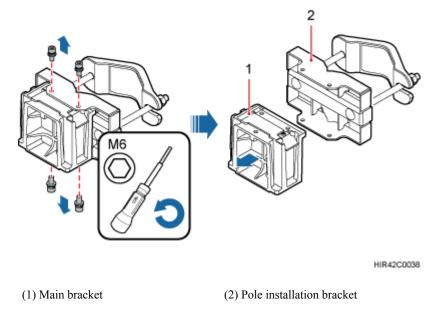
Step 3 Install the removed main bracket on one side of the first main bracket, as shown in Figure 8-10.
