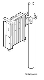
Figure 3-7 A single RRU installed on a pole
