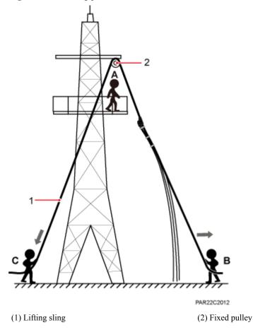
Figure 7-9 Hoisting power cables onto the tower
