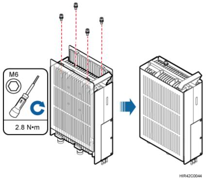
Figure 6-3 Installing the plastic shells of the RRU
