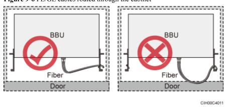
Figure 9-6 FE/GE cables routed through the cabinet
