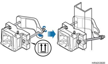
Figure 8-22 Installing the RRU mounting brackets
