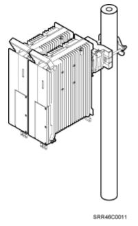
Step 2 Use an M6 inner hexagon screwdriver to remove the four inner hexagon screws from the second set of mounting brackets, and remove the main bracket from the auxiliary bracket, as shown in Figure 8-15.
