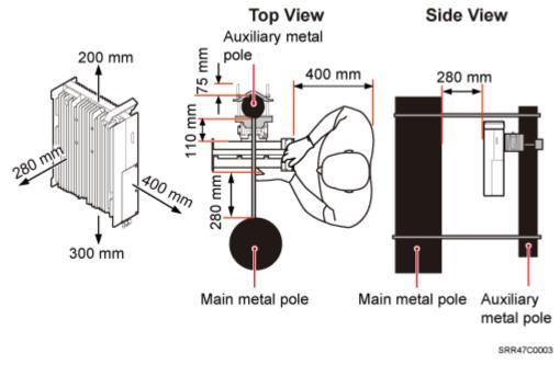
Figure 3-24 Minimum clearance for a single tower-mounted RRU in standard or reverse mode
