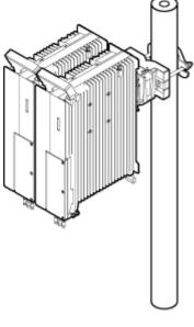
Figure 3-8 Two RRUs installed on a pole
