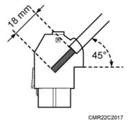
Step 4 Add a tool-less female connector (pressfit type) to two core wires.
