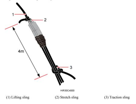
Figure 7-7 Binding fiber optic cables
