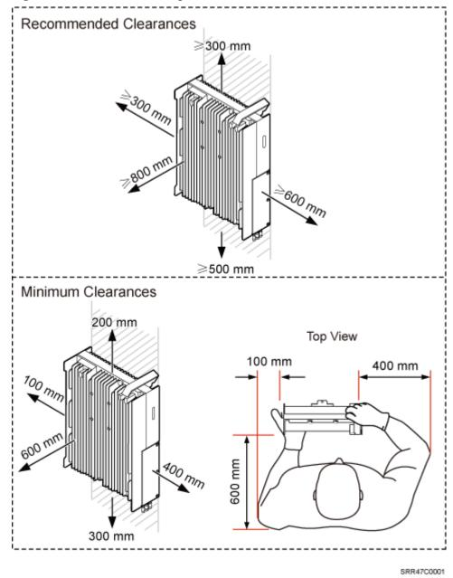
Figure 3-22 Clearances for a single RRU in standard or reverse mode
