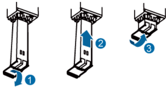
Figure 7-23 Installing an optical module
