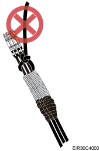
Figure 7-8 Incorrect binding method
