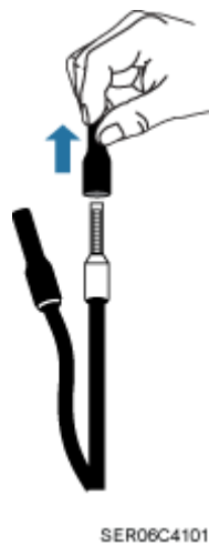
Figure 9-22 Removing insulated protective tubes from the cord end terminals
