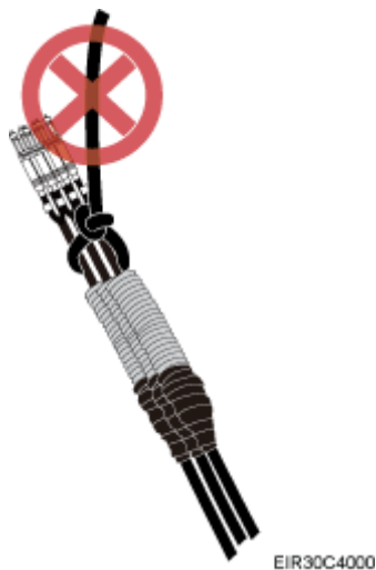
Figure 6-8 Incorrect binding method
