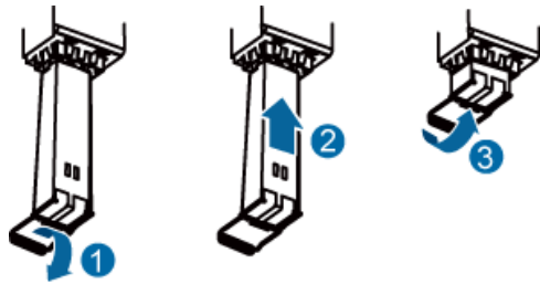
Figure 7-21 Installing an optical module
