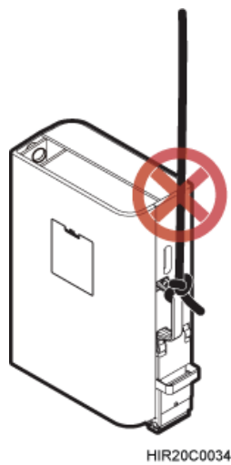
Figure 6-41 Incorrect binding method
