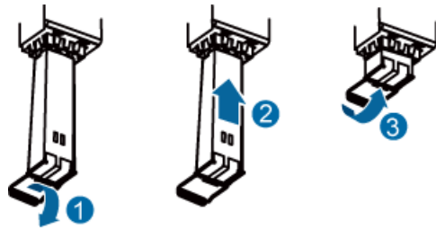
Figure 7-21 Installing an optical module
