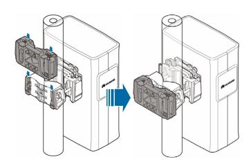
3. Reinstall the attachment plate and cover plate on the second RRU by interchanging their positions.
