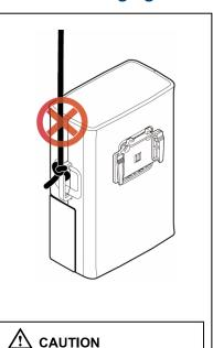
Do not bind the lifting rope
