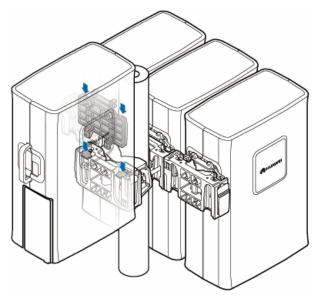
9. Four RRUs installed in centralized mode. 10. Six RRUs installed in centralized mode.
