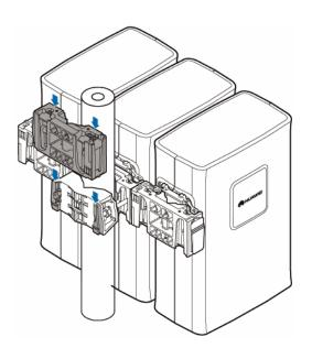
8. Fit the tabs on the attachment plate of the fourth RRU into the anchor slots on the fourth main fixture.
