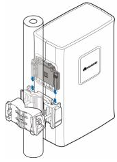
5. Fit the tabs on the attachment plate of the second RRU into the anchor slots on the second main fixture.
