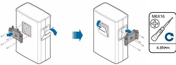
3. Fit the tabs on the attachment plate of the RRU into the anchor slots on the main fixture.
