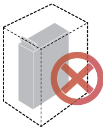
Figure 3-7 Improperly installed RRUs
