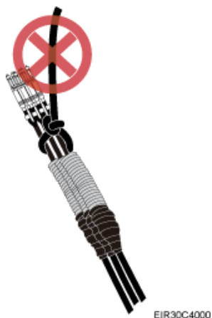
Figure 7-8 Incorrect binding method
