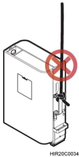
Figure 6-3 Incorrect binding method
