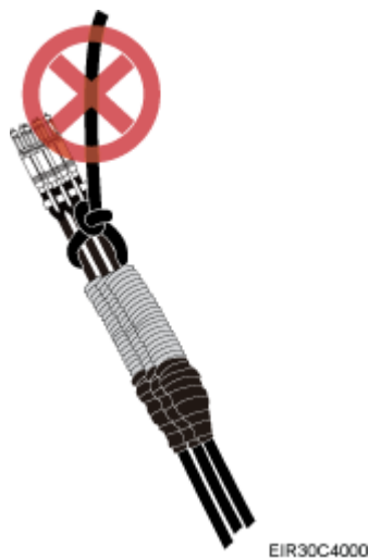
Figure 6-7 Incorrect binding method
