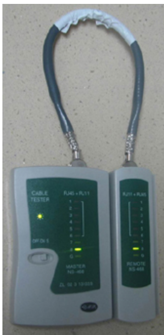
Figure 1-53 Testing the conduction and connections of wires
