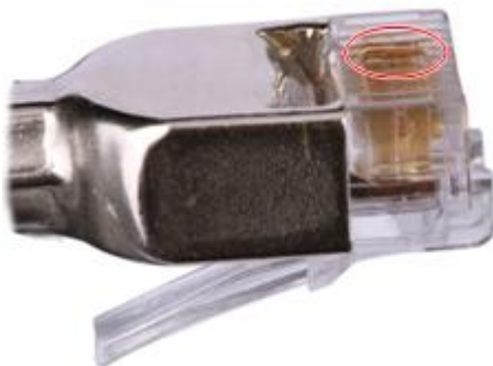
Figure 1-48 Unparallel metal contact strips of different heights
