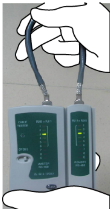
Figure 1-54 Checking the reliability
