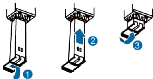
Figure 8-27 Installing an optical module
