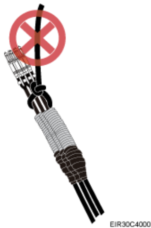
Figure 6-8 Incorrect binding method
