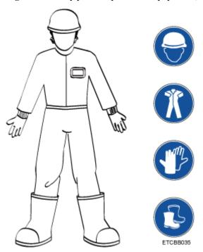
Figure 1-1 Safety personal protective equipment (PPE)
