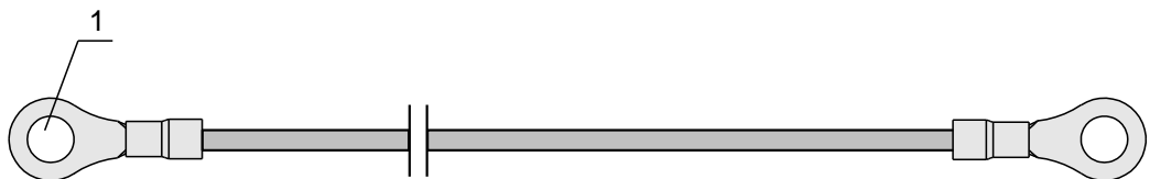
Figure 7-4 RTN 360 PGND cable
