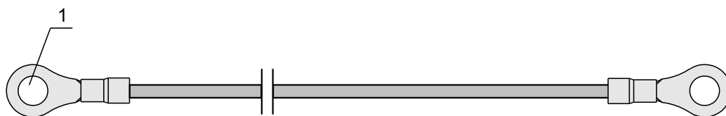
Figure 7-5 RTN 360 PGND cable
