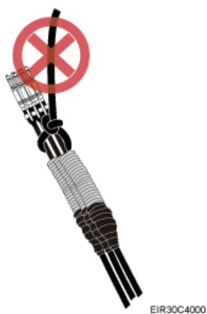
Figure 7-8 Incorrect binding method
