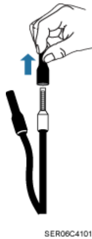
Figure 7-21 Removing insulated protective tubes from the cord end terminals
